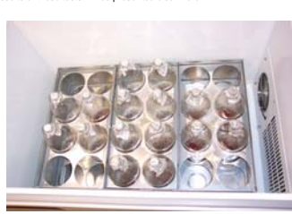
Figure 1. A photograph of the inside of a New Brunswick C25K refrigerated shaker equipped with a custom rack with capacity for up to 24 2-L PET beverage bottles used as growth vessels for bacterial cell culture.
